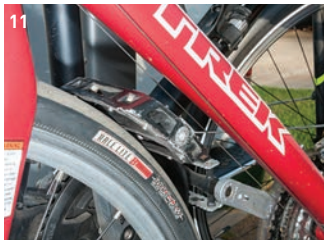
10) Cradle positions are too close for carrying four bikes. Trying to carry four bikes will likely result in damage. The rack is best suited for two bikes, although three will fit with cradle repositioning. 11) It's best to space out the cradles to prevent damage to the bike's frame from pedals or other components. 12) U-shaped ZipStrips are used to snug the bicycle frame to the cradles. 13) A ratcheting mechanism holds the ZipStrips tightly.
