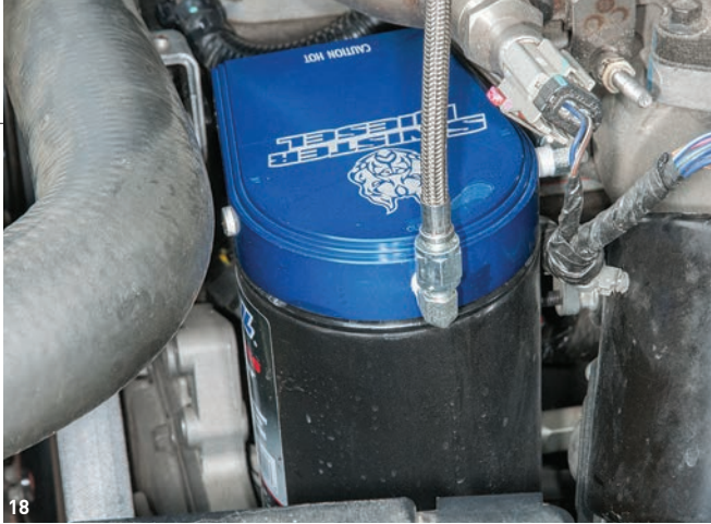
18) The Sinister filter block fits neatly next to the intake manifold, leaving enough room to install the Amsoil bypass filter after adding a quart of oil. 19) The new cap is installed, and the braided line is attached to fittings in the cap and filter block.
