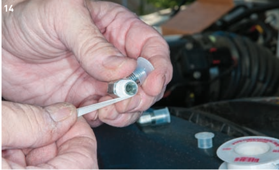
14) Teflon tape is applied to all the fittings before installing in respective locations.
