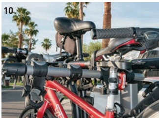
10) Cradle positions are too close for carrying four bikes. Trying to carry four bikes will likely result in damage. The rack is best suited for two bikes, although three will fit with cradle repositioning. 11) It's best to space out the cradles to prevent damage to the bike's frame from pedals or other components. 12) U-shaped ZipStrips are used to snug the bicycle frame to the cradles. 13) A ratcheting mechanism holds the ZipStrips tightly.
