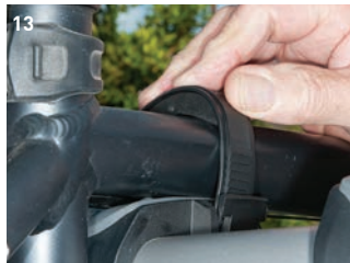
10) Cradle positions are too close for carrying four bikes. Trying to carry four bikes will likely result in damage. The rack is best suited for two bikes, although three will fit with cradle repositioning. 11) It's best to space out the cradles to prevent damage to the bike's frame from pedals or other components. 12) U-shaped ZipStrips are used to snug the bicycle frame to the cradles. 13) A ratcheting mechanism holds the ZipStrips tightly.
