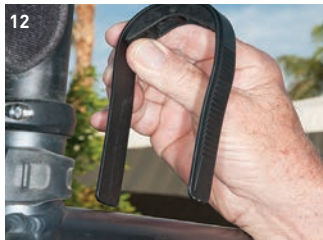
10) Cradle positions are too close for carrying four bikes. Trying to carry four bikes will likely result in damage. The rack is best suited for two bikes, although three will fit with cradle repositioning. 11) It's best to space out the cradles to prevent damage to the bike's frame from pedals or other components. 12) U-shaped ZipStrips are used to snug the bicycle frame to the cradles. 13) A ratcheting mechanism holds the ZipStrips tightly.
