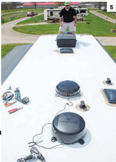
[5] Before permanently installing the Connect dome, place it on the roof to determine if it meets Winegard’s clearance requirements. It must be 12 inches from the edges of the roof and at least 12 inches away from other accessories and appliances. Power connection, SIM card slot and reset button must face the rear of the motorhome.
