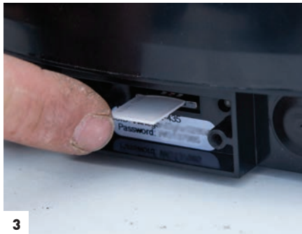
[1] Winegard Connect 2.0 4G2 4G LTE + WiFi Extender is packaged with power cable and extension, hardware kit and roof entry plate. [2, 3] If a SIM card from AT&T or Verizon is desired, it’s best to slide it into the provided slot before installing the dome on the roof. A proprietary SIM card for 4G LTE data service is installed in the slot from the factory; it must be activated for use. [4] Pertinent encryption and password information is on a tag stuck to the bottom of the dome, but will be difficult to access once the Connect is attached to the roof. The information is also on the instruction manual, which should be saved.
