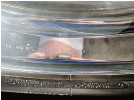
[Above, left] The factory stamping shows the maximum weight, size and inflation pressure limits for this particular wheel. These figures should never be exceeded. Installing larger tires and/or tires with higher load ranges does not mean the rim can be overloaded. When buying new tires, ensure they are properly sized for the motorhome's rims. [Above, right] This wheel is stamped AccuRide. According to the manufacturer's website, it's an uncoated wheel that's safe for traditional polishing with products made for aluminum wheels.
