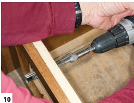
[9] Always measure twice before cutting. [10 and 11] Predrill all of the woodwork before reinstalling the mounting screws. [12] Proper installation of the new SMEV required a bit of patient manipulation, as the new configuration of space was rather snug.
