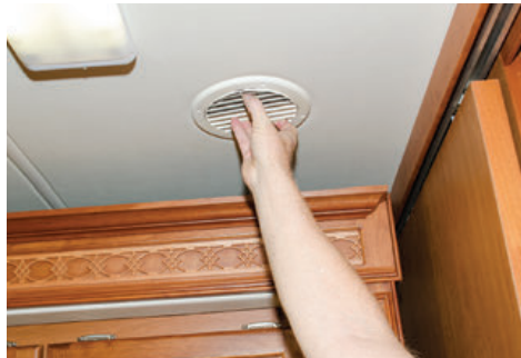
Above: Make sure to remove and clean (or replace) the HVAC return air filters before the season starts. These things can collect a shocking amount of dirt and dust, so clean and dry them completely (if cleanable), or replace with new ones, if necessary. Tire pressure should be checked before every trip. After sitting all winter, the tires should be inspected for damage, bulges and cracking, and should be inflated properly.
