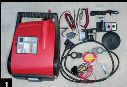
[1] BrakeBuddy kit includes everything needed to install the components on a dinghy vehicle — even additional wire.
