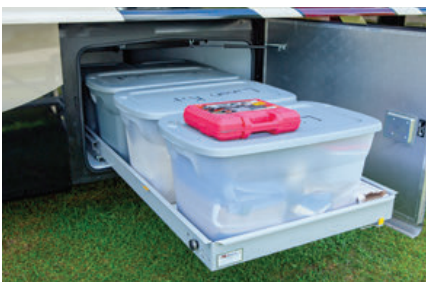
From above: Dining table can be pulled out and two chairs added to accommodate four people. Slide-out storage tray facilitates access to front compartment.
