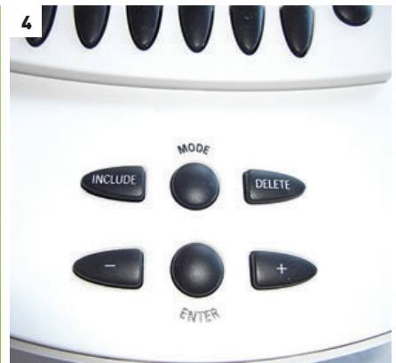
[1] This Z-Wave remote controller can turn lights and appliances on or off when they are networked with Z-Wave control modules. [2] Incandescent lamp control modules such as this one can include a dimming feature. [3] This control can relate action events to time or the on/off buttons can be used. [4] The include button on the control is pressed and held while the control module is set to program mode.
