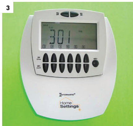
[1] This Z-Wave remote controller can turn lights and appliances on or off when they are networked with Z-Wave control modules. [2] Incandescent lamp control modules such as this one can include a dimming feature. [3] This control can relate action events to time or the on/off buttons can be used. [4] The include button on the control is pressed and held while the control module is set to program mode.
