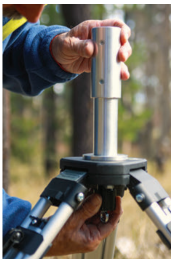
Below from left: Set the degrees of elevation and this custom aiming scope will enable you to check for obstructions in the line of sight. A solid aluminum machined mast is designed to fit a 2- or 1-5/8-inch bracket as well as supporting up to 35 pounds. The heavy-duty tripod has an infinite amount of adjustment for each leg, thus making the leveling process fast and easy.
