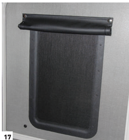
[16] The Clear View window shade is unique in that it installs on the screen, not the entry door. [17] During the day, the shade can be easily rolled up and snapped into place, or removed and stored in a cabinet. [18] The shade is held in place at each corner by a pair of strong magnets (one on either side of the screen) that are attracted to each other. They effectively secure the shade without damaging the screen.
