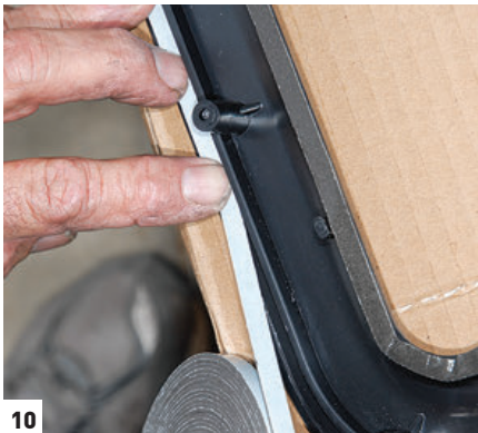
[7 and 8] Pull gently while removing the original inner and outer sealing tape to prevent leftover pieces. [9] Gently remove the original glass from the outside frame. [10 and 11] Install the new inner and outer seals, taking extra care not to damage the delicate material around the corners. [12] Set the new glass against the bottom stops and use your fingers to center the glass for a final installation.
