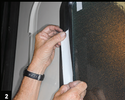
[1] The Clear View entry-door window kit comes packaged to prevent damage during shipping. [2] Use high-quality duct tape to ensure adhesion and prevent accidents. [3] When removing the inside frame, have a helper hold the outside frame and glass assembly.
