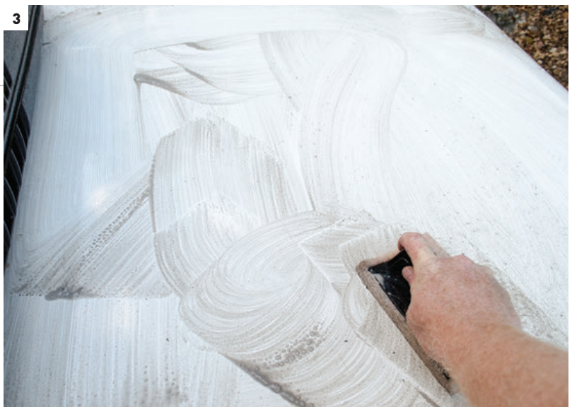
[1] After a year of sitting outside, the roof on this coach was in need of some serious cleaning. Notice the black dirt as well as the green mold toward the front. If your coach is covered with leaves and other debris you will first need to remove the offending parties by sweeping or blowing them off with a leaf blower before you begin. [2] To get started, spray a small 2-by-2-foot area with the Belly Wash, making sure the area is completely covered before you begin scrubbing. The red-colored Wash Wax All Degreaser is safe for plastics and clear-coat paint, but the purple Belly Wash shown here is not. Make sure you use each product as directed. [3] After spraying the area with Belly Wash, use the Aero Scrubber and start scrubbing. You will see the dirt and grime start to dissolve quickly. Usually it takes two or three minutes of scrubbing per area to get it clean.
