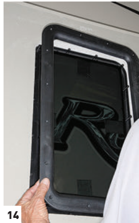
[13] Use duct tape to hold the glass and outer frame in place for a one-person job. [14 and 15] Install the inside frame top side up and do not overtighten the screws. The plastic frame will certainly crack when overtightened.
