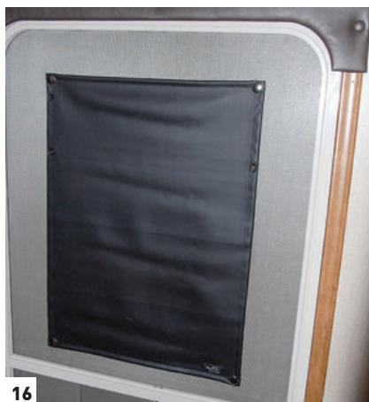
[16] The Clear View window shade is unique in that it installs on the screen, not the entry door. [17] During the day, the shade can be easily rolled up and snapped into place, or removed and stored in a cabinet. [18] The shade is held in place at each corner by a pair of strong magnets (one on either side of the screen) that are attracted to each other. They effectively secure the shade without damaging the screen.
