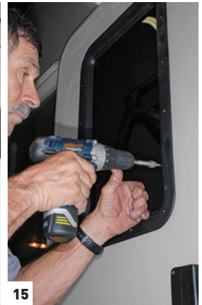
[13] Use duct tape to hold the glass and outer frame in place for a one-person job. [14 and 15] Install the inside frame top side up and do not overtighten the screws. The plastic frame will certainly crack when overtightened.
