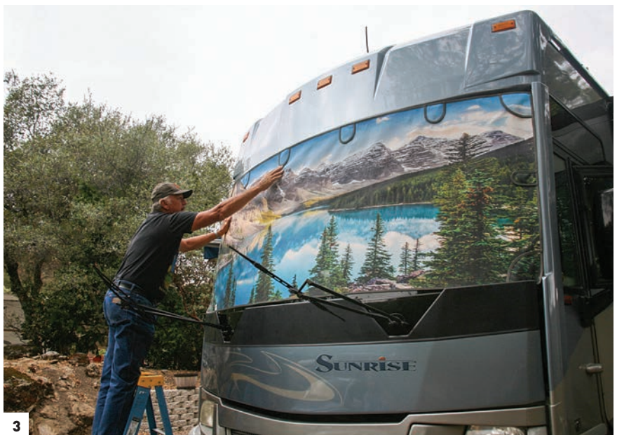
[1-3] The shade is held in place while magnets are positioned on inside surface of windshield.
