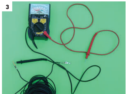
[1] A 10-watt bulb should read about 0.8 ohms resistance. [2] With the negative probe grounded, a fuse should read 12 volts DC on both sides. In this case, the fuse is blown so the meter reads 0 volts on the downstream side. [3] Along with a multimeter, a long wire with alligator clips on both ends is needed for testing ground connections.
