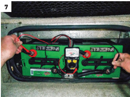
[7] Use the voltmeter function of the multimeter to verify that the battery or bank of two 6-volt batteries (shown) is charged; a fully charged battery will test at 12.7 volts. [8] Check the battery negative (-) post-to-cable connection by using the ohmmeter function of the meter, with one lead on the battery post and the other on the cable connector. [9] At the beginning of every season, detach the connection cables and clean with a wire brush.
