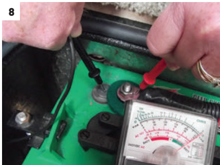
[7] Use the voltmeter function of the multimeter to verify that the battery or bank of two 6-volt batteries (shown) is charged; a fully charged battery will test at 12.7 volts. [8] Check the battery negative (-) post-to-cable connection by using the ohmmeter function of the meter, with one lead on the battery post and the other on the cable connector. [9] At the beginning of every season, detach the connection cables and clean with a wire brush.
