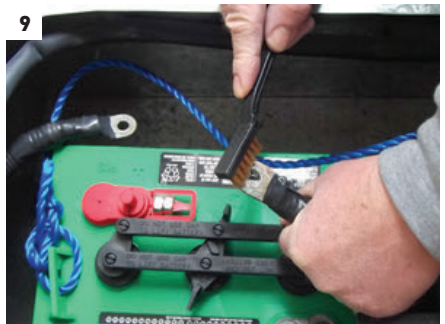
[7] Use the voltmeter function of the multimeter to verify that the battery or bank of two 6-volt batteries (shown) is charged; a fully charged battery will test at 12.7 volts. [8] Check the battery negative (-) post-to-cable connection by using the ohmmeter function of the meter, with one lead on the battery post and the other on the cable connector. [9] At the beginning of every season, detach the connection cables and clean with a wire brush.
