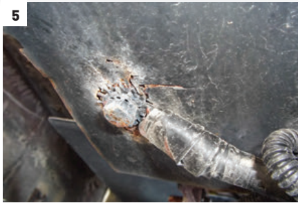
[4] A 12-volt DC circuit breaker should read about 0 ohms. [5] The heavy negative battery cable should be properly grounded to the frame. Oxidized or frayed connections like this one should be repaired even if they test OK to prevent troubles down the road. [6] (illustration) An example of a simple direct-current circuit.
