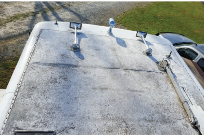
Above from left: On this old, neglected motorhome roof, the decking is buckling under the membrane. There's no sealant left on the extrusion around the outside of the roof. Television and radio antennas, air horns and roof-termination seams are among the locations where sealants should be examined and reapplied on a regular basis.
