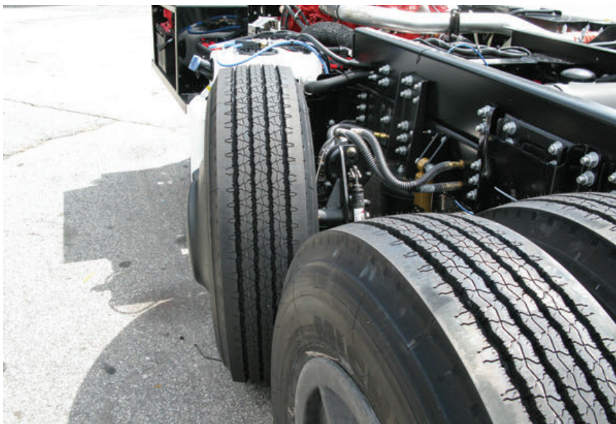
Steering tag axle is designed to reduce curb-to-curb turning radius by 17 percent, improve handling and limit tire scrubbing.
