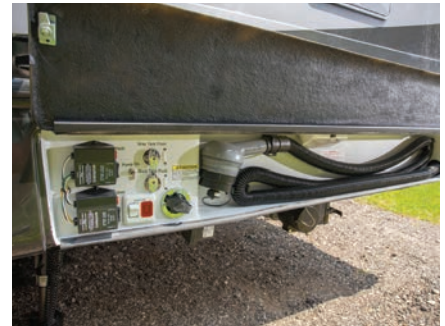
Rear storage locker is a welcome feature that can handle larger items. Ladder to roof folds up to allow the door to swing open. The utility bay is well thought out and is fitted with electric dump valve controls, gray- and black-water flush hookup, and a Thetford macerator pump and hose.
