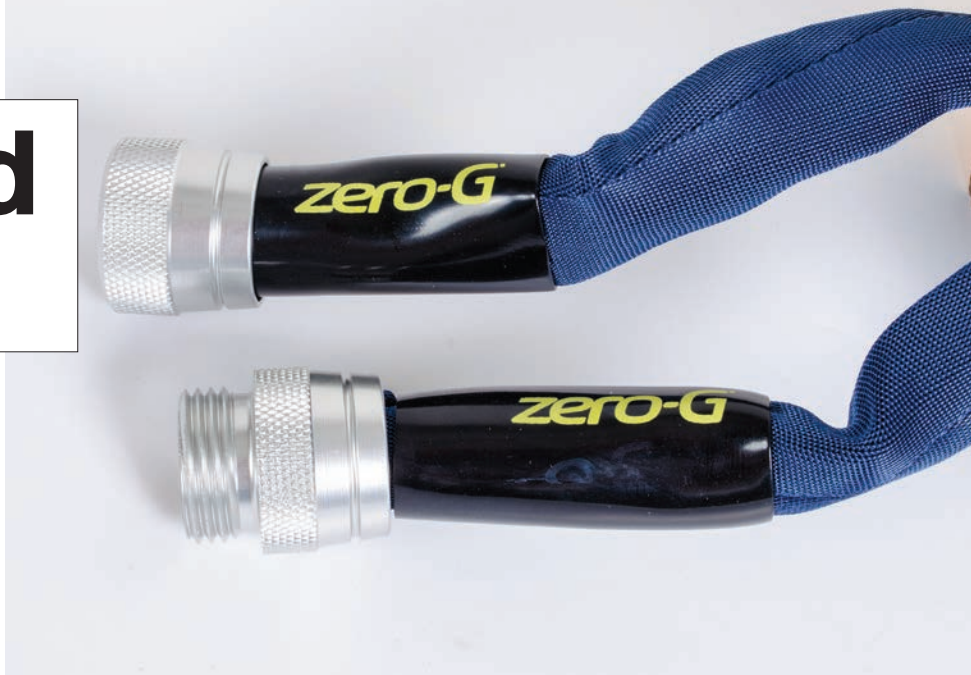
Above: Each end of the hose has a strong rubber collar to reinforce the connection point, and knurled aluminum fittings for ease of use.
