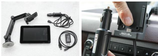
Above left: Mounting hardware and cables (power and for downloading upgrades) are provided with the kit. Above right: An articulating arm with suction cup holds the mounting bracket firmly to the windshield. The plug goes into a nearby 12-volt DC accessory power port.
