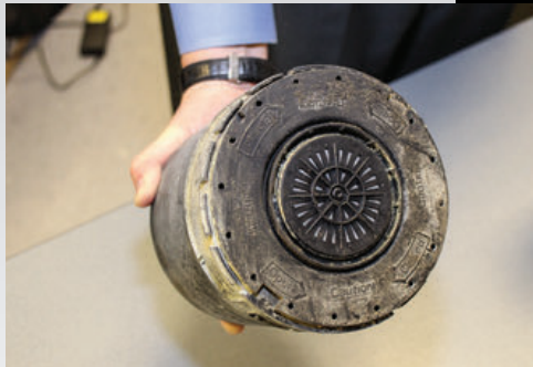
Far left: An abused air filter, blocked by an animal nest, caused severe engine damage. Left: Ignoring the air dryer can also have catastrophic consequences. Here's an air dryer cartridge that has failed, and the desiccant has come out of the element. This allowed excessive moisture to collect in the air system, requiring replacement of most of the system, costing thousands of dollars. Below: An FCCC-certified factory technician checks the ride height on a customer's motorhome.
