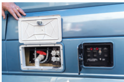
Sewage disposal and tank flushing (left) is easy with the macerator system with electric reel. The driver's compartment (right) is luxurious and comfortable. Note the matching painted panels.
