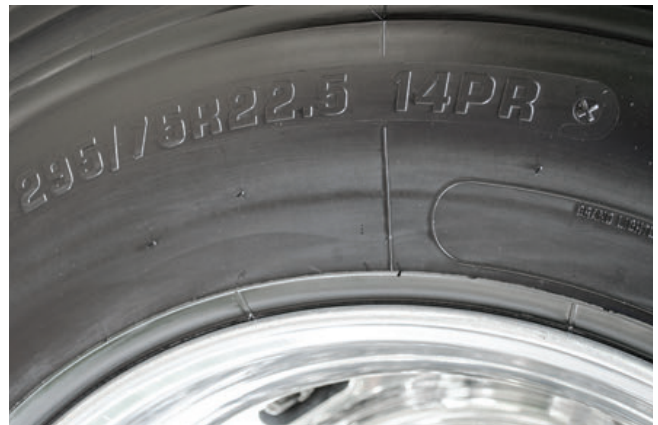
Above: In order to determine the correct inflation pressure for a motorhome's tires, you need to know the size and load range of tires installed on the coach. That info is shown here on the sidewall of the tire.
