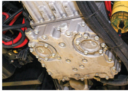
Above: Changing the fuel filters (above left) should be done at every oil change, according to Cody. The Allison transmission has two circular filter cartridges — shown here on the bottom of the transmission pan. Follow the maintenance schedule for service intervals based on your particular model transmission. An important element in maintaining the air system is bleeding air from the system. Pictured here are two halyards (above right) that when pulled, open valves in the air tanks to release accumulated moisture. These should be pulled open daily for 15 seconds while traveling, unless your coach is equipped with automatic bleeders, in which case once per month should suffice. A third halyard should be at the rear of the chassis.
