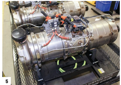
[3, 4] The Selective Catalytic Reduction (SRC) system converts nitrogen oxides into harmless nitrogen and water using urea, which is stored in a separate tank (inset). The newest version [5] combines all the components (VOC, DPF and SCR) into one space-saving canister, also allowing the full cleaning procedure to be extended to between 600,000 and 800,000 miles.
