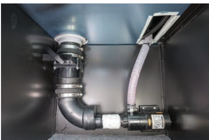
Above: The Vista's cockpit (left) is comfortable and is afforded great views from the one-piece windshield. The first black-tank valve (right) feeds into a macerator in a compartment on the passenger side.
