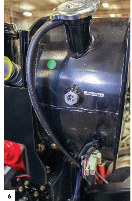
[6] Spartan uses a coolant reservoir that has a window to show the level of the coolant. The color makes it easy to see, but is not a true indication of condition, so the coolant should be changed according to the maintenance schedule for the chassis.
