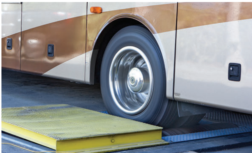
Measuring power at the drive wheels results in real-world numbers directly relating to performance you get on the road.
