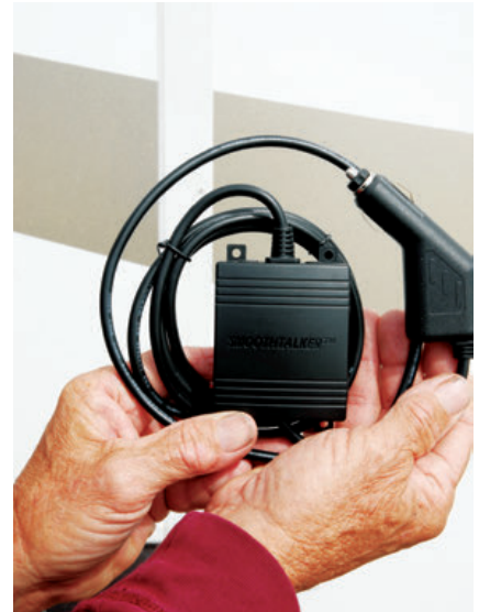
Users who choose not to hardwire the booster to 12-volt DC power can use an optional power supply that plugs into an accessory port.
