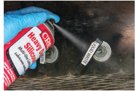
Periodically clean and lubricate the holding-tank valve handles and cables to keep them operating smoothly.
