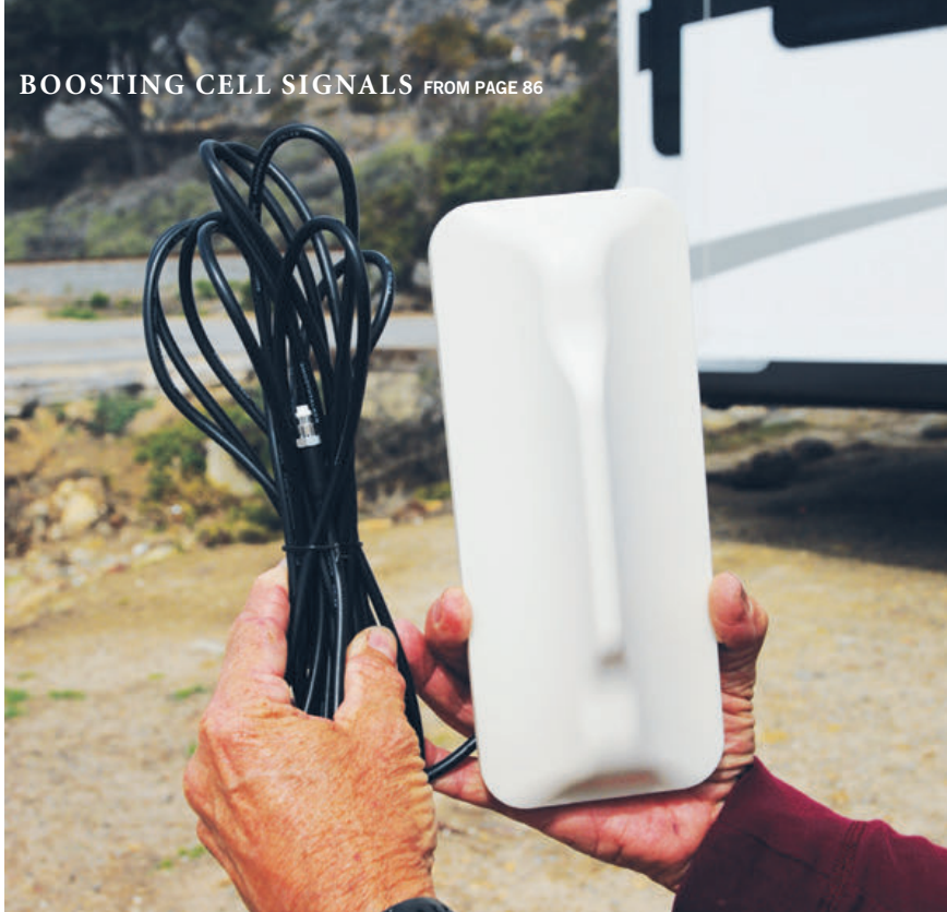
Wideband High Gain Directional Antenna improves service when in fringe areas, and can be used inside RVs that are too short for optimum separation from the outside antenna.
