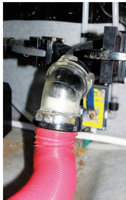
A clear plastic elbow is attached to the pipe to which a sewer hose can be connected so the user can see what is being flushed.
