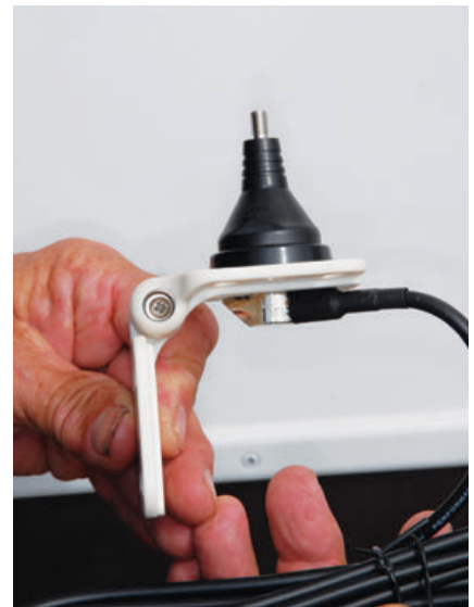
Clever bracket is designed to facilitate antenna mounting to a rear ladder or even the side wall of the motorhome.
