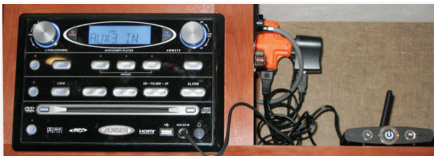
Above: Ancillary components to power the Miccus receiver/transceiver and hook up to the stereo are included in the kit. Below: Unit is placed inside a cabinet next to the stereo and connected via a 1/8-inch auxiliary port.
