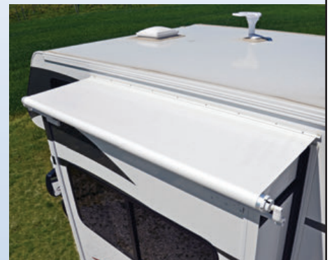
SlideToppers shield the tops of slideouts against moisture, debris and direct sunlight.
