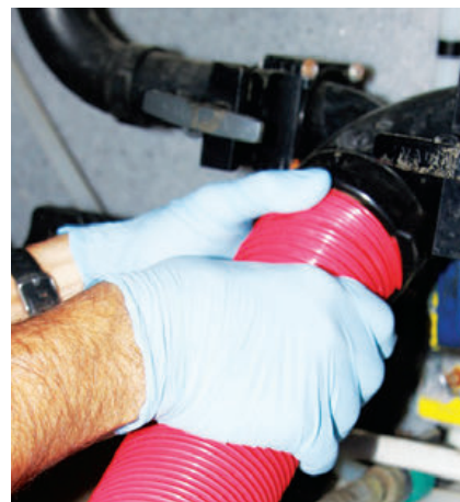
Sewer hose is attached to the motorhome in preparation for emptying the tanks at a dump station.
