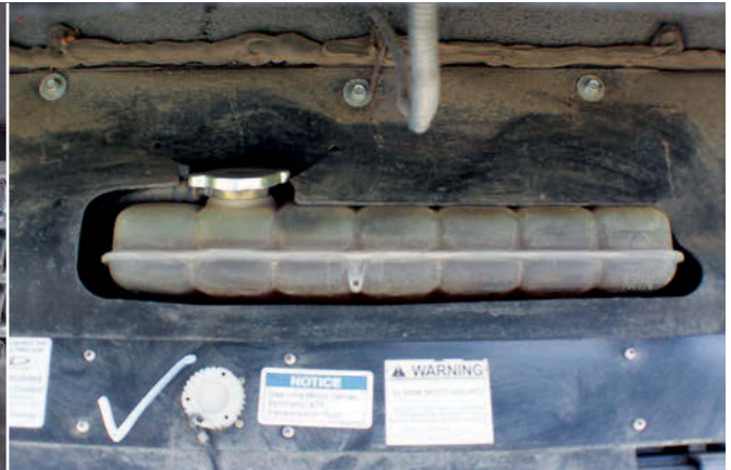
Earlier-model diesel-pushers incorporated the radiator cap directly on top of the coolant overflow tank.
