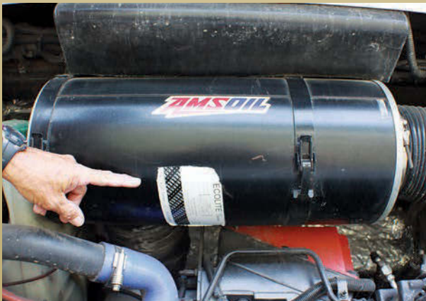
Many diesel-pushers have a sealed air filter located within a metal canister that is easy to access inside the engine compartment.
