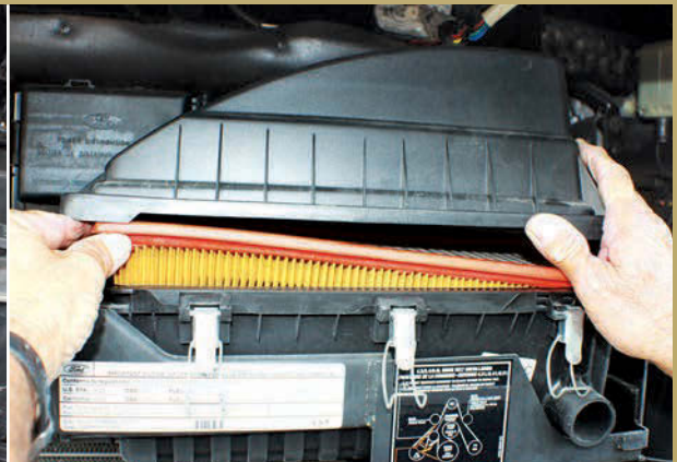
To get to the filter element, unlatch the housing and pull up the top portion to gain access. It's best to keep a record of filter changes and check visually during service.
