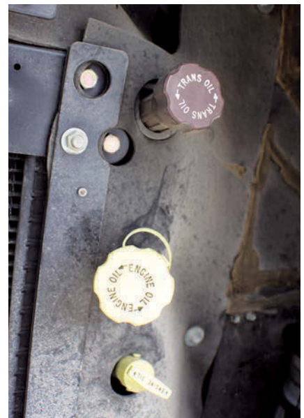
It is important to check transmission fluid level in diesel-pushers and gas chassis. This particular chassis model positions the transmission and engine oil dipsticks together in a convenient location.
