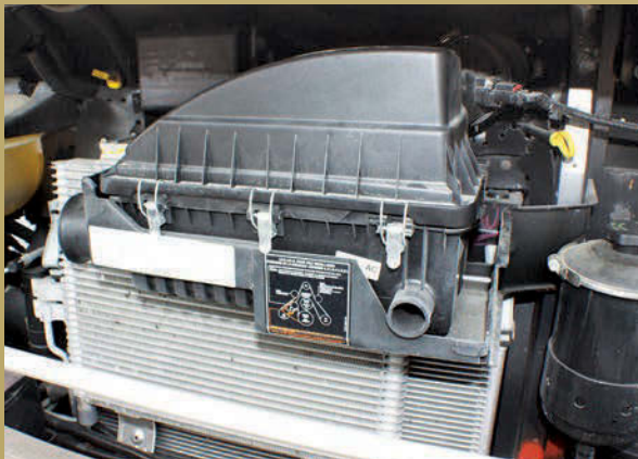
Most Class A motorhomes with gas powered engines are fitted with a housing that uses a replaceable air filter element.
