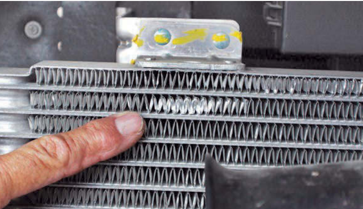
Over time, radiator fins can become damaged, thus adversely affecting the overall cooling capacity. A fin-straightening tool will make short work out of realigning bent fins.
