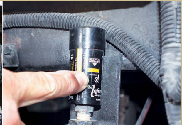
It is imperative to check the overflow restriction gauge, which takes the guesswork out of filter service.
