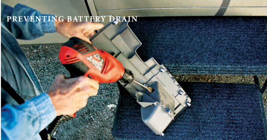
Check clearance and drill a 3/4-inch hole in the lower dash panel coin pocket.
