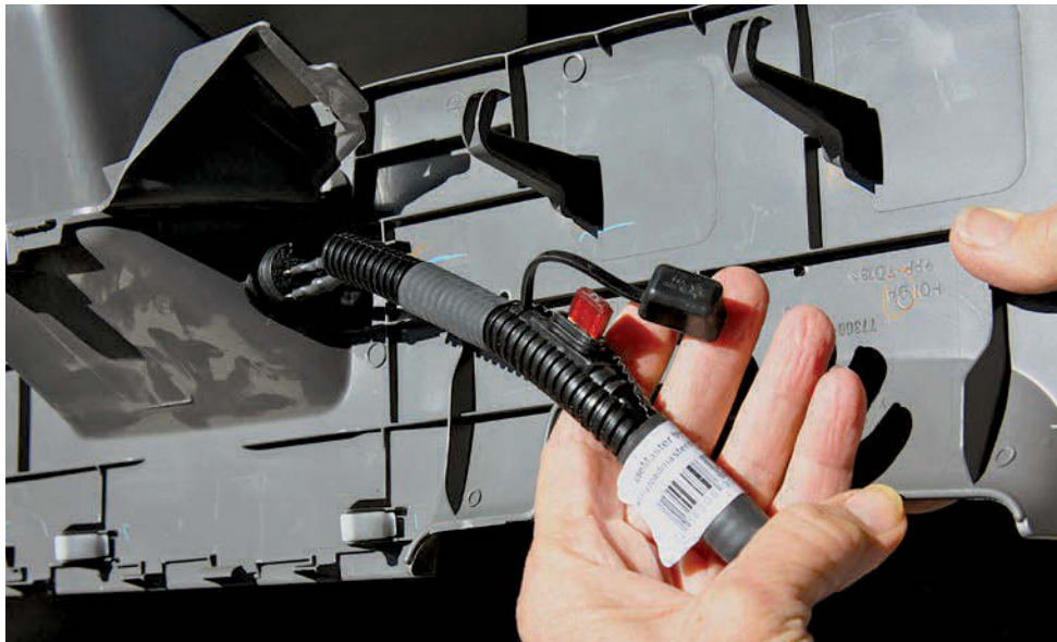
Position the harness in the lower dash panel.
