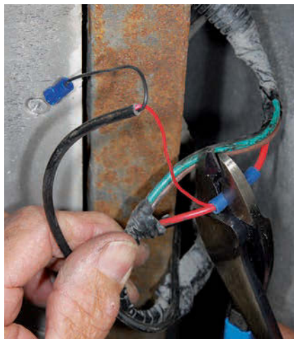
When tapping into the reverse wire of the coach, we chose to use a butt connector, rather than the supplied Scotchlok, as the butt connector offers a longer-lasting connection. A steel cross member made a convenient spot for the ECU ground wire.
