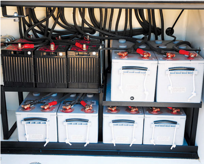
Banks for big motorhomes can include multiple starting batteries and a number of 4D gel-cell batteries to power coach systems.
