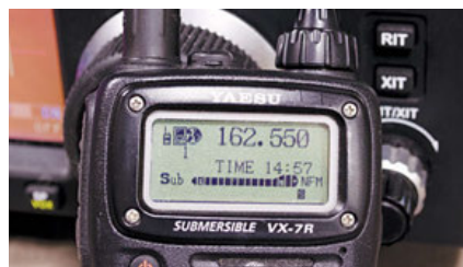
One safety feature of the VX-7R Yaesu radio is its built-in access to all NOAA weather bands for instant access to weather information.
