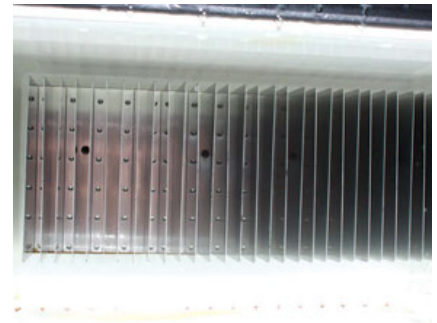
Be sure the refrigerator's interior cooling fins are intact and evenly spaced for maximum cooling output.
