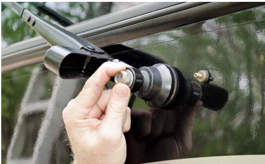
After the arm is in place and level, reinstall the washer and nut on the threaded drive stud and tighten.
