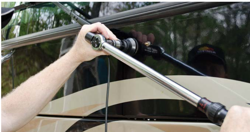
The manufacturer of this particular wiper arm (TRU Vision) recommends that the new arm be torqued twice to ensure it is properly seated. Then reconnect the washer fluid hose and you are ready to move to the other side and repeat.
