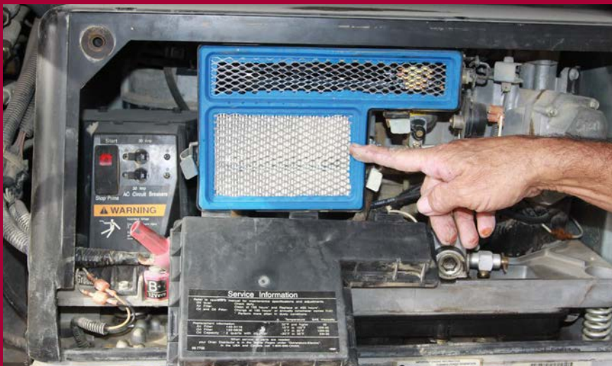
The Onan Marquis Models air filters are easily accessible from behind the main generator cover.
