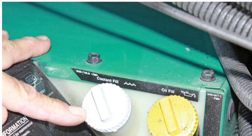
The Onan Quiet Diesel models provide easy access for checking oil and anti-freeze levels.
