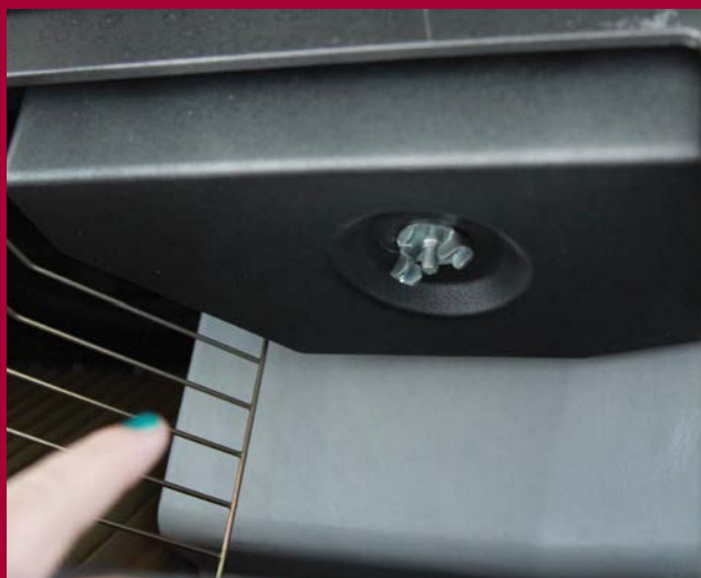
The air filter of the Onan 4.0 kW Microquiet is accessible by removing a single wing nut and cover.
