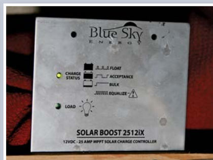
The Solar Boost 2512iX charge controller can increase charge current up to 30 percent or more.
