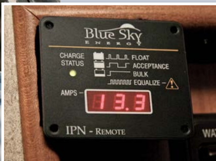
This monitor from Blue Sky displays battery voltage, output current and charge control system status.
