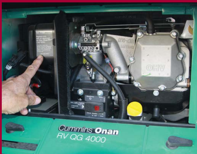
The air filter of the Onan Quiet Diesel, which requires access from underneath the generator, is still easily accessible for servicing.
