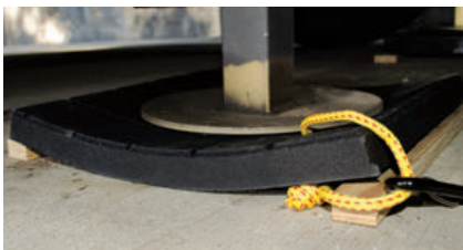
The Hosspad is designed to bend and conform to difficult subgrades and showed no signs of stress after this test.
