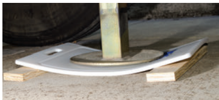
The cutting board may work well on flat concrete or asphalt but don't expect it to bridge difficult subgrade conditions or prevent the jack feet from sinking into soft soil or sand. From our tests these are best left in the kitchen.
