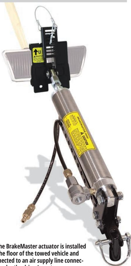
⬆ The BrakeMaster actuator is installed on the floor of the towed vehicle and connected to an air supply line connector under the driver's seat.
