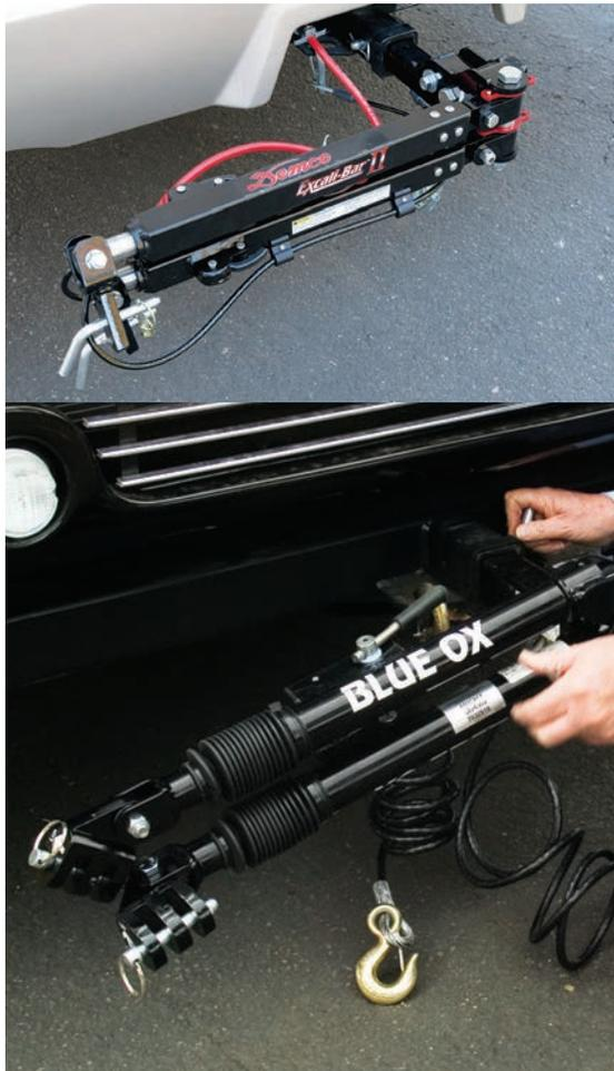
⊖ While driving the dinghy, this type of tow bar remains on the motorhome. ⊕ Once the tow bar is pinned in the hitch receiver, ensure the electric connections and safety cables are secure.
