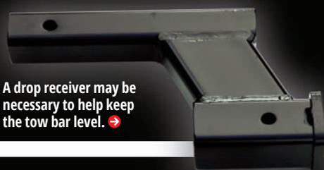
A drop receiver may be necessary to help keep the tow bar level. ➔
