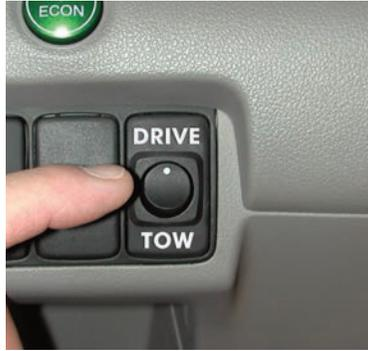
**FuseMaster kit eliminates the need to pull a fuse before towing the dinghy vehicle, then reinserting after disconnecting. Simply flipping a switch accomplishes the same task.**
