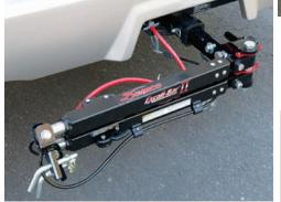
Above: Once the tow bar is pinned in the hitch receiver, make sure electric connections and safety cables are secure. Left: While driving the dinghy, this type of tow bar remains on the coach, out of harm's way.
