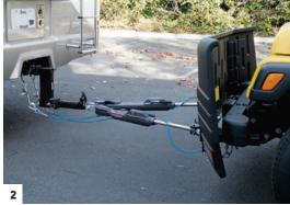
Coach-mounted units are the most desirable, as there is less chance of damage when not in use — and hitching is a one-person operation. Highly adaptable, self-aligning tow bars fit a broad range of vehicles by attaching to model-specific baseplates: Class III (5,000-pound) or Class IV (10,000-pound) models are available. Contact tow-bar manufacturers to find out if baseplates are offered for the dinghy you plan to tow.
