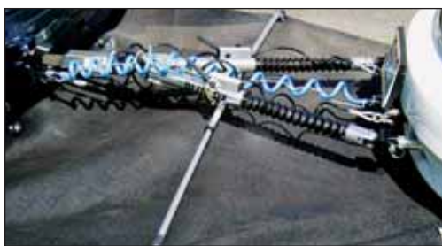
AN RV UNDERSKIRT WILL KEEP TOWING APPARATUS CLEAN — AND IT ALSO HELPS PROTECT THE FRONT OF THE TOWED VEHICLE FROM ROAD DEBRIS.
