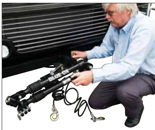
ONCE THE TOW BAR IS ATTACHED TO BOTH VEHICLES, MAKE SURE ELECTRIC CONNECTIONS AND SAFETY CABLES ARE SECURE.
