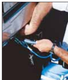
PLUG RECEPTACLES ADDED TO DINGHY AND MOTORHOME ALLOW EASY HOOKUP OF ELECTRICAL CONNECTOR FOR TAILLIGHTS, TURN SIGNALS AND SUPPLEMENTAL BRAKING SYSTEM.
