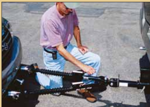
ONCE THE PINS ARE IN, THE MOTORHOME IS DRIVEN AHEAD SLOWLY (OR DINGHY BACKED) TO LOCK THE ARMS IN POSITION.
