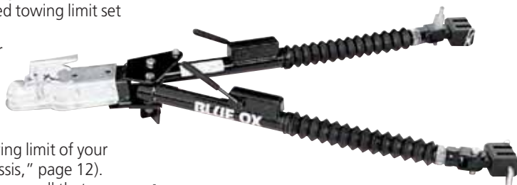
A BALL COUPLER ON A TOW BAR LOOKS SIMILAR TO THAT ON A TYPICAL TRAILER A-FRAME.
