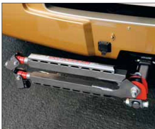
WHILE DRIVING YOUR DINGHY, THIS TOW BAR REMAINS ON THE COACH, TUCKED OUT OF HARM'S WAY.
