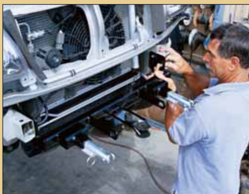
BASEPLATE INSTALLATION DOES NOT REQUIRE WELDING OR SPECIALIZED TOOLS, BUT CAN BE INVOLVED. IF YOU HAVE ANY DOUBTS, HAVE A PROFESSIONAL DO IT.
