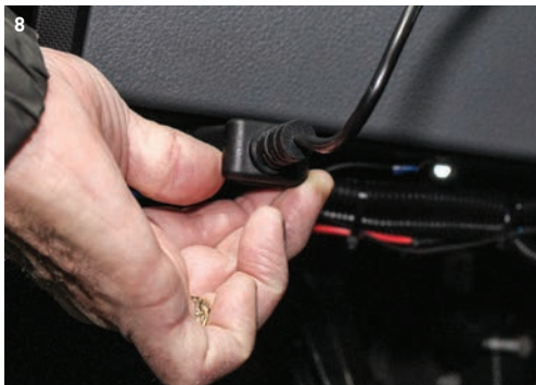
8) The 5-Star programming device plugs in to the vehicle's OBD-II port and can be left connected so it acts as a customizable digital-gauge readout. 9) The dynamometer control station shows all the vehicle data in real time and records the numbers for later analysis. The computer will immediately create charts showing vehicle performance. 10) A 5-Star Tuning technician shows the hand control for the dynamometer that he uses while running the tests from inside the truck.
