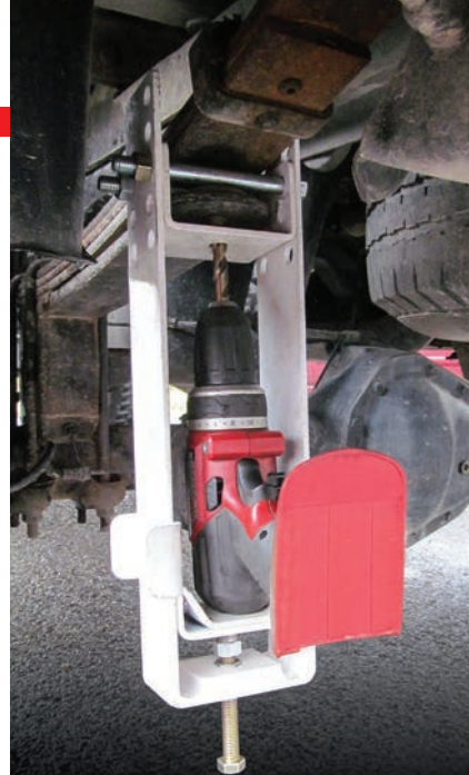
7) A \frac{3}{8} -inch ratchet and extension are used to engage the Quick Disconnect stabilizer. 8) A clip and pin keep it in place in the engaged position.
