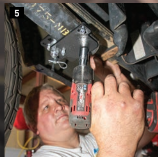
4) The StableLoad Quick Disconnect stabilizers are assembled with three wedges to fit the gap between the lower overload spring and the main leaf springs. 5) A 7/16-inch bolt secures the wedge pack to the overload spring. The bolt is torqued to 35 lb-ft. 6) The wedge pack is set in the disengaged position.
