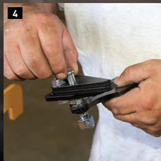
4) The StableLoad Quick Disconnect stabilizers are assembled with three wedges to fit the gap between the lower overload spring and the main leaf springs. 5) A 7/16-inch bolt secures the wedge pack to the overload spring. The bolt is torqued to 35 lb-ft. 6) The wedge pack is set in the disengaged position.
