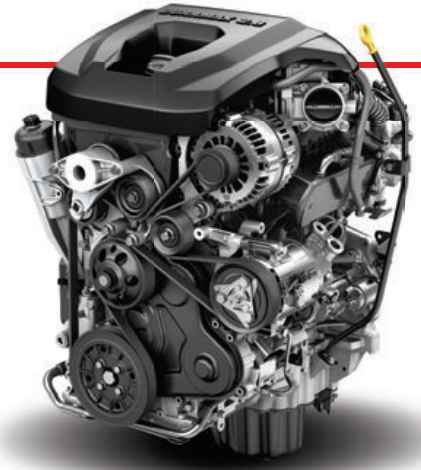
Chevy Colorado and GMC Canyon will offer a 2.8-liter Duramax diesel that should top 30 mpg highway and tow at least 7,000 pounds.
