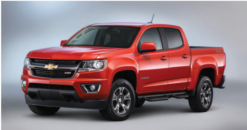
Chevy Colorado and GMC Canyon will offer a 2.8-liter Duramax diesel that should top 30 mpg highway and tow at least 7,000 pounds.
