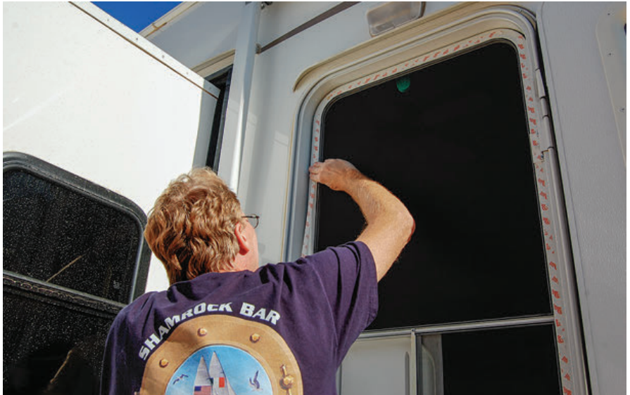
A screen door can be made winter ready with the use of an inexpensive window-insulation kit. The project takes about an hour.
