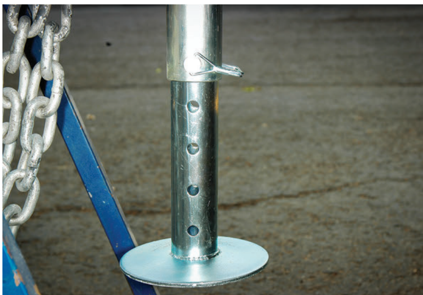
(Top) The key-fob-style remote for controlling the electric jack shaves a lot of time off the hitching and leveling processes. (Above) An adjustable extension adds 6 inches to the 18-inch leg provided by the electric jack.
