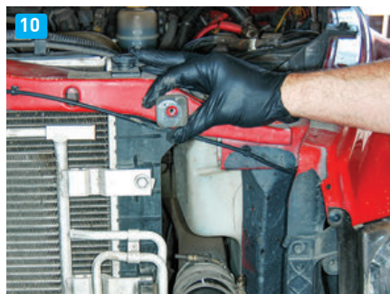
[7] Access to the clamps holding the passenger-side boot is a little tight but can be handled easier with air tools. [8] The upper bolts that secure the factory intercooler are removed. [9] Once the bolts are removed, the factory intercooler can be pivoted up from the lower U-shaped isolators. [10] The two upper rubber isolators are retained and installed on the new BD Cool-It intercooler.
