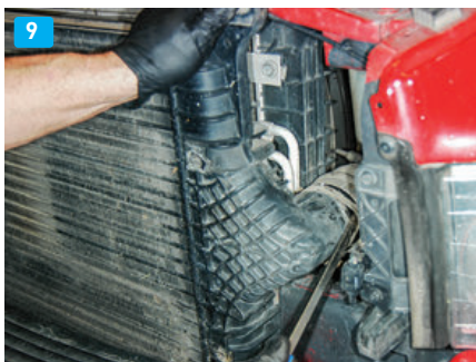
[7] Access to the clamps holding the passenger-side boot is a little tight but can be handled easier with air tools. [8] The upper bolts that secure the factory intercooler are removed. [9] Once the bolts are removed, the factory intercooler can be pivoted up from the lower U-shaped isolators. [10] The two upper rubber isolators are retained and installed on the new BD Cool-It intercooler.
