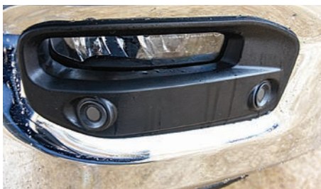
Ⓢ ParkSense sensors are now mounted in plastic instead of in the steel bumper, which reduces the likelihood of freezing.
