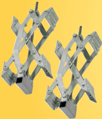
Ultra Super Grip Chock, Set of 2 Eliminates front-to-back rocking motion when applied between tandem trailer tires, using opposing force.
