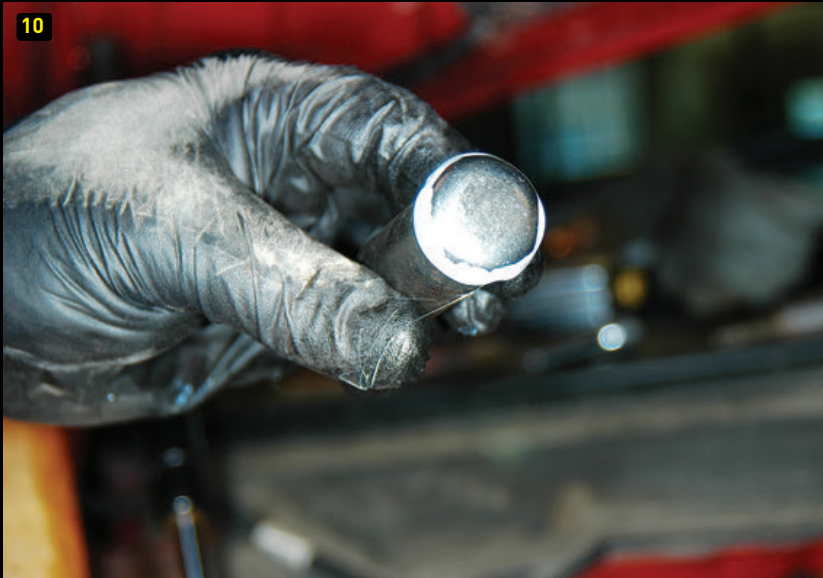
(10) Sealant is spread on the new freeze plug before installing in the cylinder head.
