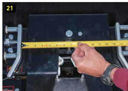
(19) With the pivot head in place, the release handle is installed with the supplied nut and bolt. (20 and 21) Carefully measure the pin box and then set the guides on the pivot head for a tight fit.
