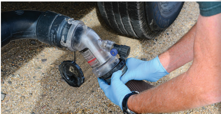
(Above) A clear plastic elbow is attached to the pipe on the trailer to which a sewer hose can be connected so the user can see what is being flushed. (Right) The sewer hose runs from the RV to the dump-station.
