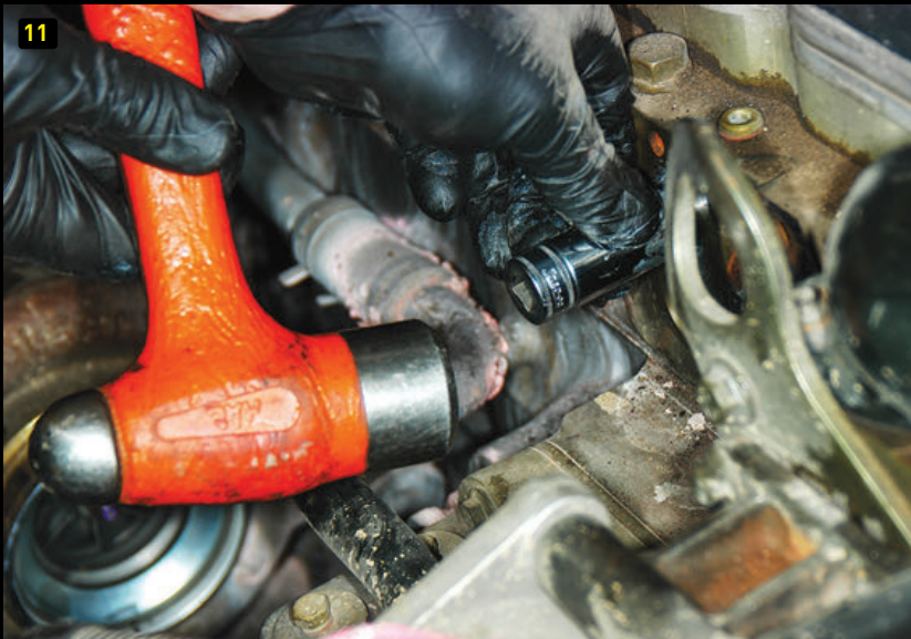
(11) An old ratchet socket is used to pound the new freeze plug into position, creating a pressed fit.
