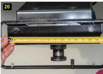
(19) With the pivot head in place, the release handle is installed with the supplied nut and bolt. (20 and 21) Carefully measure the pin box and then set the guides on the pivot head for a tight fit.
