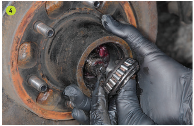
(1) Carefully pry the dust cap from the hub and drum assembly. Excessive damage may cause the dust cap to become dislodged during travel. (2) Remove the cotter pin that holds the spindle nut in place. After servicing, always use a new cotter pin. (3) Remove and replace the spindle nut using a large pair of adjustable pliers. (4) Be careful not to drop the outer bearing when removing the hub and drum assembly, which may damage the bearing.
