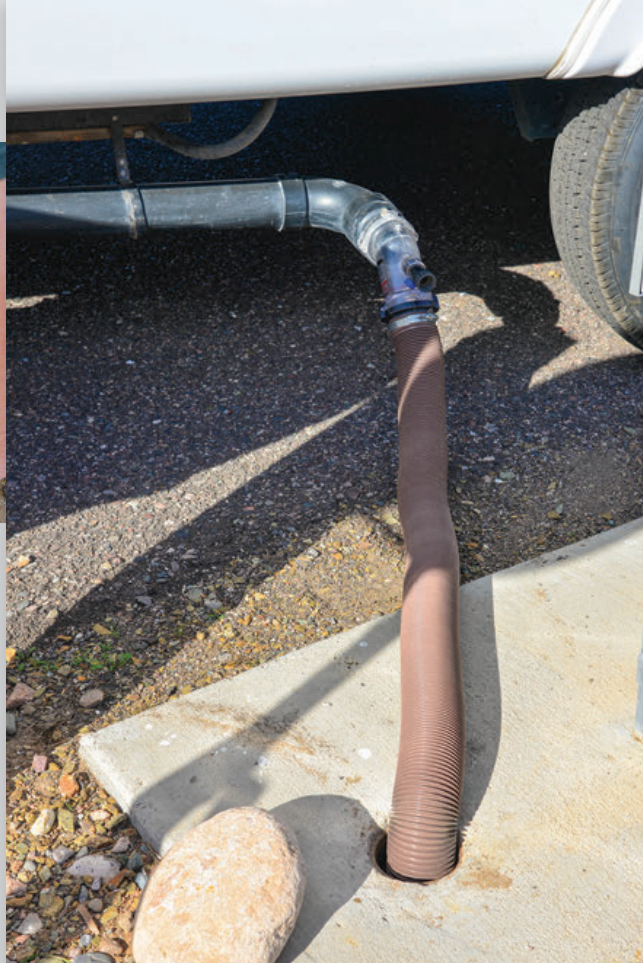
(Above) A clear plastic elbow is attached to the pipe on the trailer to which a sewer hose can be connected so the user can see what is being flushed. (Right) The sewer hose runs from the RV to the dump-station.
