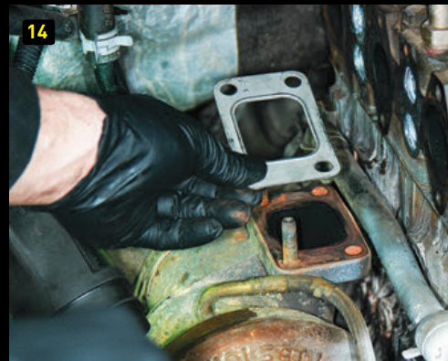
(12) New freeze plugs are in the cylinder head, which is ready for cleanup. (13) Scotch-Brite pads are used to remove all the soot and carbon buildup on the head gasket surfaces. (14) The new turbo gasket is placed on the flange; replacement studs (part of the kit) are inserted in the turbo flange.
