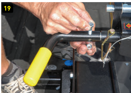
(19) With the pivot head in place, the release handle is installed with the supplied nut and bolt. (20 and 21) Carefully measure the pin box and then set the guides on the pivot head for a tight fit.
