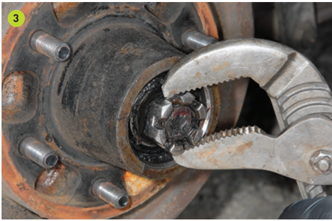
(1) Carefully pry the dust cap from the hub and drum assembly. Excessive damage may cause the dust cap to become dislodged during travel. (2) Remove the cotter pin that holds the spindle nut in place. After servicing, always use a new cotter pin. (3) Remove and replace the spindle nut using a large pair of adjustable pliers. (4) Be careful not to drop the outer bearing when removing the hub and drum assembly, which may damage the bearing.
