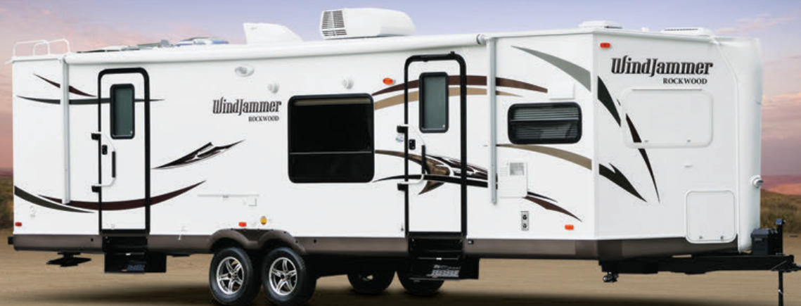
The Windjammer's marine-type V-nose shape reduces drag and wind resistance, but perhaps the most realized benefit is the extra square footage.
