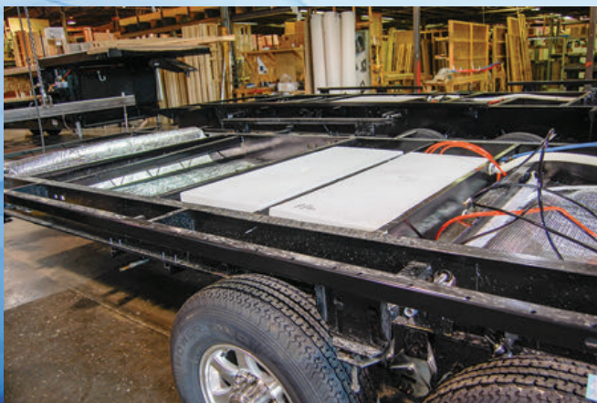
(Above from left) Typical installation of holding tanks in the chassis of a fifth-wheel trailer. How's this for a scenic dump station? This one at Deer Creek State Park in Utah has the prettiest view we've seen!
