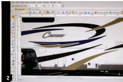
1) A digital photo of the trailer's side wall was taken with a camera and downloaded to VIP Enterprises' special computer-graphics program. 2) This is done to generate a pattern for the new vinyl graphics. 3) Close-up detail on the screen allows the operator to create a precise pattern. At this point the customer can ask the designer to make changes to the pattern to suit his or her taste.
