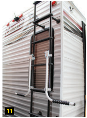
10, 11, 12) The arms lock straight out for carrying the tank and to the outsides for climbing the ladder. When the tank isn't mounted, the arms remain unlocked, folded inward and strapped down. 13) The tank is secured to the ladder with the included cinch-strap. It sits nicely on the bracket, with tabs on the tank (inset) that help secure it to the arms.
