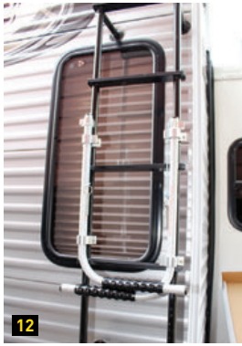
10, 11, 12) The arms lock straight out for carrying the tank and to the outsides for climbing the ladder. When the tank isn't mounted, the arms remain unlocked, folded inward and strapped down. 13) The tank is secured to the ladder with the included cinch-strap. It sits nicely on the bracket, with tabs on the tank (inset) that help secure it to the arms.
