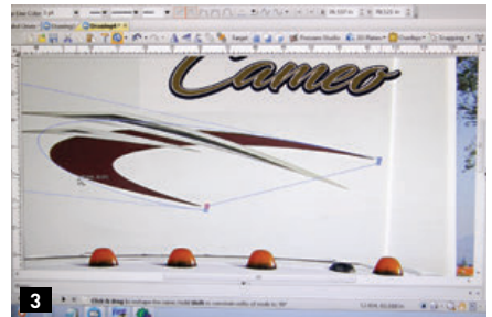
1) A digital photo of the trailer's side wall was taken with a camera and downloaded to VIP Enterprises' special computer-graphics program. 2) This is done to generate a pattern for the new vinyl graphics. 3) Close-up detail on the screen allows the operator to create a precise pattern. At this point the customer can ask the designer to make changes to the pattern to suit his or her taste.
