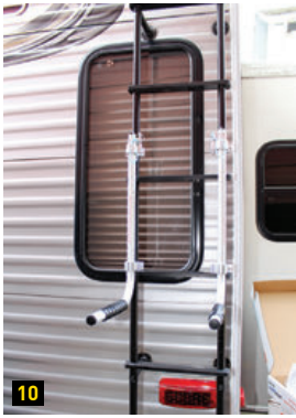
10, 11, 12) The arms lock straight out for carrying the tank and to the outsides for climbing the ladder. When the tank isn't mounted, the arms remain unlocked, folded inward and strapped down. 13) The tank is secured to the ladder with the included cinch-strap. It sits nicely on the bracket, with tabs on the tank (inset) that help secure it to the arms.
