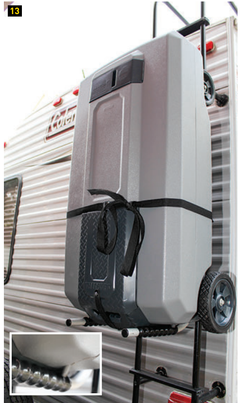
10, 11, 12) The arms lock straight out for carrying the tank and to the outsides for climbing the ladder. When the tank isn't mounted, the arms remain unlocked, folded inward and strapped down. 13) The tank is secured to the ladder with the included cinch-strap. It sits nicely on the bracket, with tabs on the tank (inset) that help secure it to the arms.
