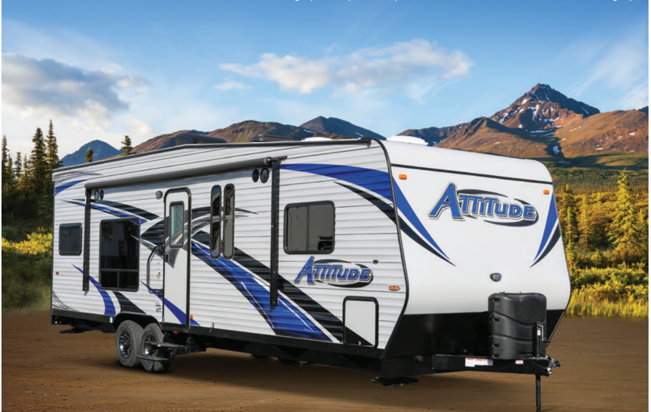
The Attitude's standard exterior uses hung aluminum panels with a lighter touch of graphics. Fiberglass siding is optional.
