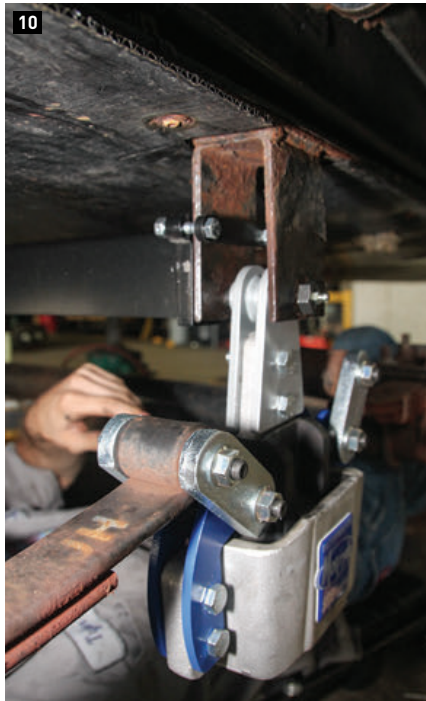
10) The X-Factor cross member is mounted to the spring hanger, and the equalizer is fully mounted with the thicker shackles. 11) The SRE4000 system is completely installed. Note that the only zerK fitting facing out is the one at the top of the equalizer. The other fittings face in, so they can be accessed and greased without removing the tires and wheels.
