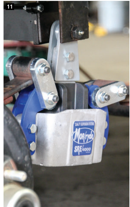
10) The X-Factor cross member is mounted to the spring hanger, and the equalizer is fully mounted with the thicker shackles. 11) The SRE4000 system is completely installed. Note that the only zerK fitting facing out is the one at the top of the equalizer. The other fittings face in, so they can be accessed and greased without removing the tires and wheels.
