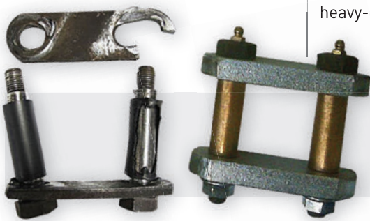
Thin shackle plates and nylon bushings can deteriorate over time, allowing the bolt holes to elongate and eventually wear all the way through (far left). MORryde's heavy-duty upgrade (left) includes thicker plates, bronze bushings and zerk fittings. The kit, or similar components, should be standard equipment.
