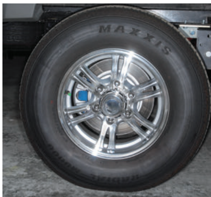
(Above left) Checking window and door seals for signs of wear is equally important. Reseal, if needed, trying to match the original sealant as closely as possible and following instructions carefully. (Center) In addition to looking for cracks and wear, check the DOT date of manufacture on each tire to make sure the tires haven't exceeded the manufacturer's recommended life span. (Right) Checking for rodent infestation is another essential part of preparing a stored RV for travel. Often, because of food spills, pests will migrate to the kitchen range and nest there, or at least leave their calling card. Line this area with aluminum foil to catch spills but don't block vent holes.
