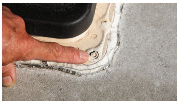
(Above) One of the most important things to do on an RV is maintain the roof seals. For warranty compliance, some manufacturers require that they be inspected every 90 days and resealed as needed. (Top) Be sure to use the proper sealant for the brand and type of roof. Failure to do so can result in hidden leaks that can cause considerable damage over time.
