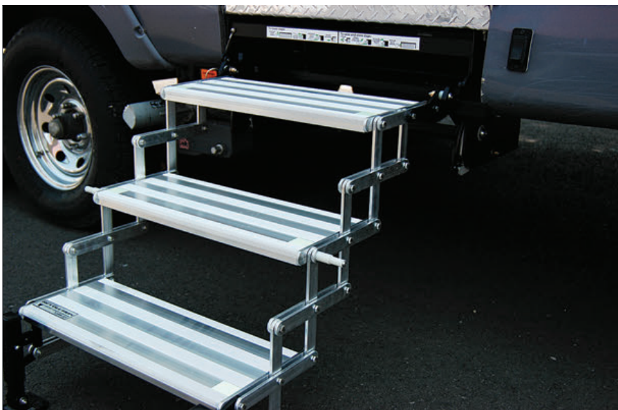
The near-effortless scissor-type mechanism allows the steps to be adjusted to accommodate various heights from the ground. A three-step model was installed on the test trailer; systems are also available with two, four, five or six steps.
