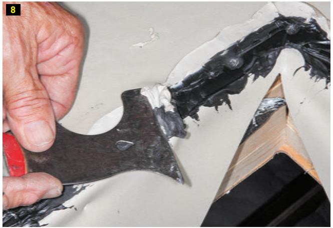
(7) The original roof vent is lifted off the roof. In this case the sealant was pretty fresh, so it was messy to work with. (8) A scraping tool is used to remove excess sealant from the rubber membrane surrounding the hole in the roof. Go slowly and use caution to prevent cutting the membrane.
