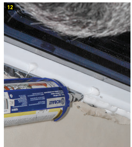
(9) A foam gasket is applied to the Fan-Tastic Vent before it is positioned (10) into the hole in the roof. No other sealant is needed on the gasket surface. (11) Once it has been established that the fit is correct (from the inside) and the shroud slides into place without restriction, it's time to attach the new vent to the roof using the supplied screws. (12) Lap sealer is applied around the edges of the Fan-Tastic Vent frame and on the screw heads. Lap sealer fills voids as it spreads. It takes a little practice to apply the right amount of sealer; in most cases, more is not better.
