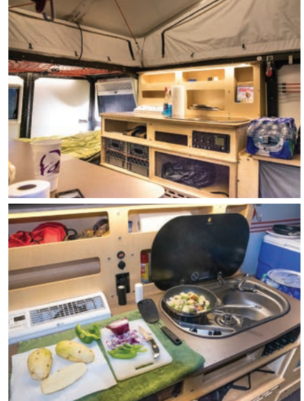
Made from marine-grade birch plywood, the galley houses a two-burner Dometic stove-and-sink combo and offers more than enough counter space for meal prep.
