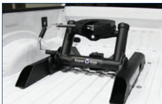
BXR6200: fits any 2-5/16" gooseneck hitch ball
