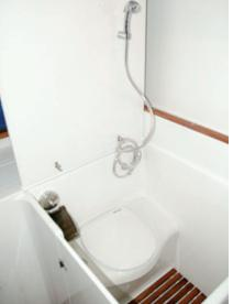
(Far left) The efficient Dometic Coolmatic compressor refrigerator does not need to be level like the more common absorption-type ones in most RVs. (Left) Out of sight under a hinged counter when not needed, the wet bath is actually quite large and includes a shower and Thetford cassette toilet.
