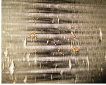
(Above, left to right) Cracks and corrosion are signs that a radiator should be replaced, ideally with a heavier-duty one. Regular maintenance of the radiator and air-conditioning condenser, including removing bugs and other baked-on debris, can help prevent overheating.
