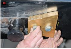
company can provide a custom-cut wedge for Sidewinder users. Once hitched, the breakaway cable can be connected to the carabiner on the end of the handle.
