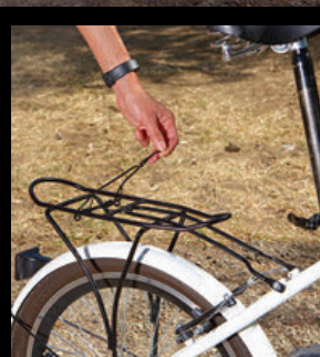
A luggage rack with a spring-loaded hold-down is designed to handle lightweight items, like a small bag or water bottle.
