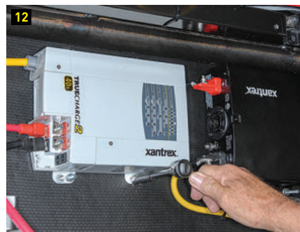
[10] RJ12 cable for the remote panel is plugged into the top position in the charger. The bottom position is for the battery temperature sensor. [11] The access cover is reinstalled on the charger after completing the wiring procedure. [12] Once wired, the charger can be installed in its permanent home.
