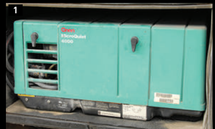
2) The Cummins Onan 4,000-watt generator is a single-cylinder, air-cooled engine designed to run on gasoline. Above the Start/Stop switch (A) is the carburetor (B), which is fitted with a mixture screw (C) at the bottom to allow limited adjustments for altitude. The cover emblazoned with "Onan OHV" is the valve cover. Bottom right is the yellow oil filler/dipstick (D). Note the large brush assembly (E); this acts as a gasket to compartmentalize the engine components when the cover is in place, promoting proper airflow from the fan (at left, not visible) over the critical engine components. It is for this reason that you should never run the generator with the cover off, even in very hot weather. Make sure you have the ID tag info (F) on hand when ordering parts.
