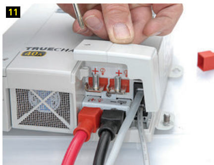
[10] RJ12 cable for the remote panel is plugged into the top position in the charger. The bottom position is for the battery temperature sensor. [11] The access cover is reinstalled on the charger after completing the wiring procedure. [12] Once wired, the charger can be installed in its permanent home.
