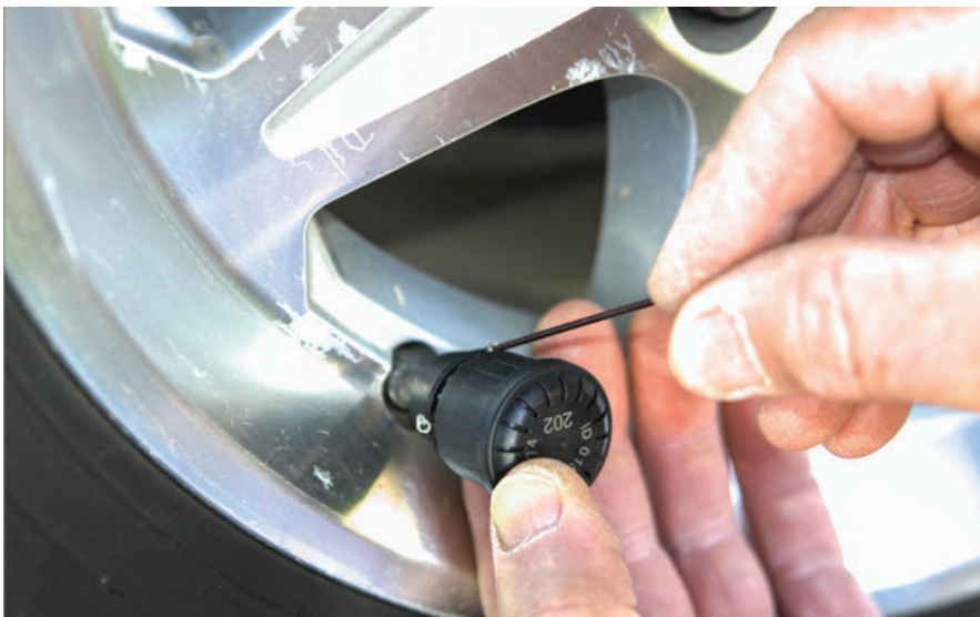
Doran's locking ring securely fastens the sensors to each valve stem.
