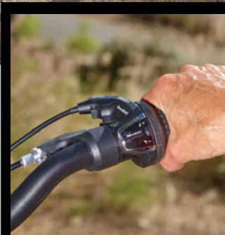
The shifter on the inside of the handlebar grip is turned to change gears.
