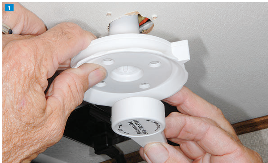
[1] The original crank mechanism in the ceiling is removed, exposing a rod, which will pull out with the batwing antenna body.
