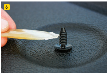
(6) Pine-tree pins are coated with rust-preventing gel that's provided with the DualLiner kit. Pushing firmly using a twisting motion drives the pins into the bed. No tools are necessary. (7) Once installed, the DualLiner makes the bed look new.
