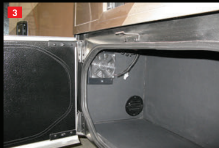
(1) Rather than using standard issue heat ducting, the Aqua-Hot relies on a network of 5/8-inch PEX tubing that's routed to individual heat exchangers. (2) Typically, a heat exchanger is installed inside the utility bay. (3) Here the backside of the heat exchanger can be serviced from inside a neighboring compartment.
