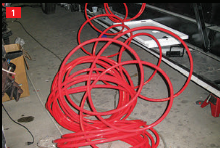
(1) Rather than using standard issue heat ducting, the Aqua-Hot relies on a network of 5/8-inch PEX tubing that's routed to individual heat exchangers. (2) Typically, a heat exchanger is installed inside the utility bay. (3) Here the backside of the heat exchanger can be serviced from inside a neighboring compartment.
