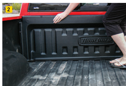
(1) Before starting the installation of the new bed liner, all the hardware, such as tie-downs, must be removed. (2) The load-guard panel, located at the front of the truck bed, is snapped into place. Positioning this panel is easy, and the fit is precise.
