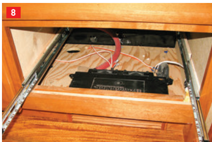
(7) Heat exchangers are strategically placed to provide the best distribution of warm air. (8) A common location for a heat exchanger is at the bottom of a cabinet drawer. (9) Switches for the system are installed in a central cabinet with other fifth-wheel controls.
