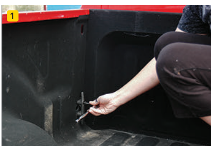
(1) Before starting the installation of the new bed liner, all the hardware, such as tie-downs, must be removed. (2) The load-guard panel, located at the front of the truck bed, is snapped into place. Positioning this panel is easy, and the fit is precise.
