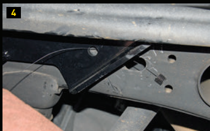
4) The piece of supplied fish wire is fed through the hole in the bracket and the corresponding hole in the frame, and then passed back out through the larger oblong hole in front of it.
