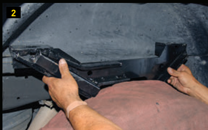
1) Part of what makes installing the PullRite ISR Series SuperRail Mounting Kit so easy is this cleverly engineered, application-specific bracket system that bolts to the frame just above the rear wheels.
