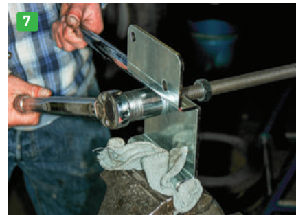
(4) Once the bumper is out of the way, it's easy to remove the spare-tire winch assembly. (5) The Titan STAFS kit comes with all the necessary hardware for installation. (6) The tank is precisely molded to fit in the area once occupied by the spare tire. (7) Minor assembly of the truck-mounting plate is accomplished using two of the large flange nuts and the presized \frac{3}{4} -inch threaded rod.
