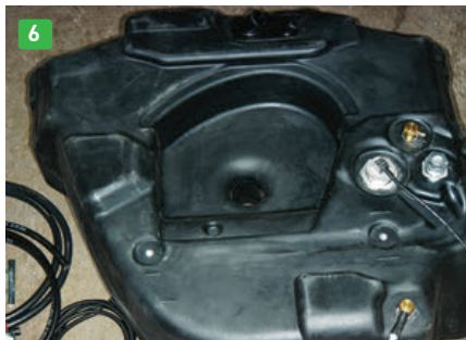
(4) Once the bumper is out of the way, it's easy to remove the spare-tire winch assembly. (5) The Titan STAFS kit comes with all the necessary hardware for installation. (6) The tank is precisely molded to fit in the area once occupied by the spare tire. (7) Minor assembly of the truck-mounting plate is accomplished using two of the large flange nuts and the presized \frac{3}{4} -inch threaded rod.
