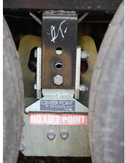
As seen in this view of the Center Point air-ride equalizer, there are limitations when servicing this type of hardware.
