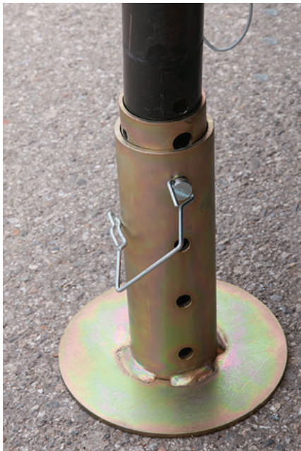
(Far left) A sizing collar is used on jack tubes that are undersized for the Quick Foot; the setscrew locks it in place. (Left) Holes in the tubing at 2-inch increments allow height adjustments from 2 to 6 inches.
