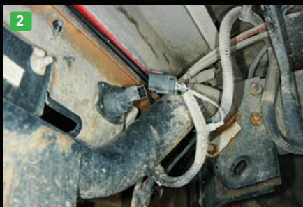
(1) The install of the Titan STAFS starts by lowering the spare tire from the rear of the truck; the tire will require storing in the truck bed. (2) Before removing the bumper, the license-plate light is unplugged. (3) Bolts are removed from the attachment brackets to release the bumper, which is set aside.
