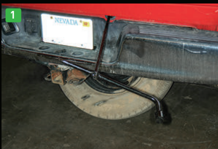
(1) The install of the Titan STAFS starts by lowering the spare tire from the rear of the truck; the tire will require storing in the truck bed. (2) Before removing the bumper, the license-plate light is unplugged. (3) Bolts are removed from the attachment brackets to release the bumper, which is set aside.
