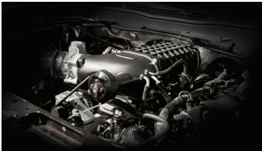
A Magnuson TVS1900 supercharger is installed on a GM 6.2-liter V-8 by Lingenfelter.
