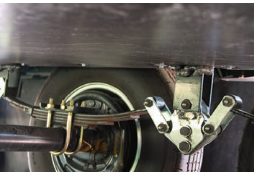
Above: (Left) This aftermarket equalizer uses a rubber carrier in the center to help smooth out some of the bumps. (Middle) Improvements in the last few years have incorporated a device that allows for correcting alignment; this particular model is called the Correct Track. (Right) Air-ride equalizers will greatly improve the ride quality, but the owners will need regular access to compressed air to sufficiently inflate the airbag to the correct pressure and, of course, there's a potential for a puncture to the airbag.
