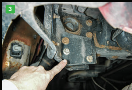
(1) The install of the Titan STAFS starts by lowering the spare tire from the rear of the truck; the tire will require storing in the truck bed. (2) Before removing the bumper, the license-plate light is unplugged. (3) Bolts are removed from the attachment brackets to release the bumper, which is set aside.
