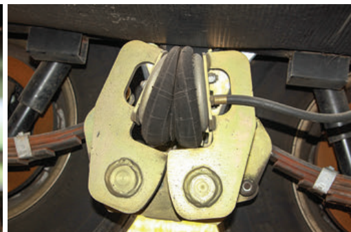
Above: (Left) This aftermarket equalizer uses a rubber carrier in the center to help smooth out some of the bumps. (Middle) Improvements in the last few years have incorporated a device that allows for correcting alignment; this particular model is called the Correct Track. (Right) Air-ride equalizers will greatly improve the ride quality, but the owners will need regular access to compressed air to sufficiently inflate the airbag to the correct pressure and, of course, there's a potential for a puncture to the airbag.
