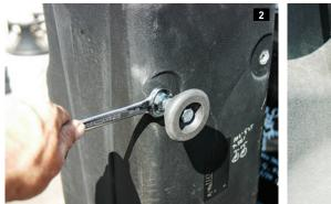
(1) The Titan Sidekick tank is lightweight and designed to mount in the little-used space in front or back of the wheel well in a pickup bed. The tank's polyethylene material is very durable and resistant to the elements. (2, 3) A bumper used to stabilize and level the tank is attached to a fitting that's molded into the material. Height is easily adjustable with a wrench. Once the bumper stop is adjusted correctly, the tank will sit level in the bed of the pickup — and feel secure.
