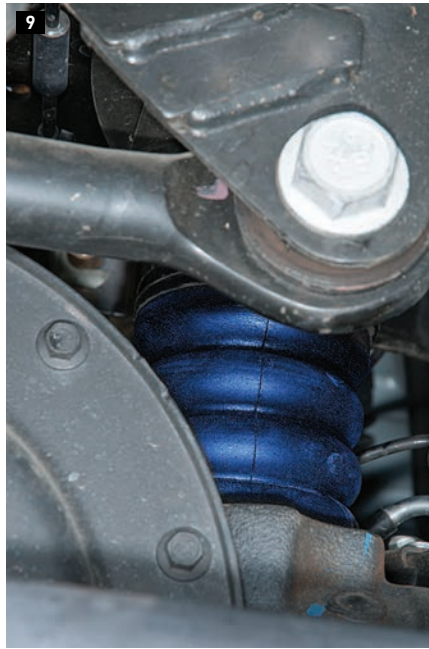
8) One-piece front spring (left) is positioned into the factory jounce bumper retaining cup. 9) Lowering the front will usually allow the spring to seat. It may be necessary to use a piece of wood to fill in the gap temporarily while seating, as was the case in the test installation (not shown). 10) The right-front factory jounce bumper (arrow) was a little more difficult to access, but it can still be done without removing the front wheels.
