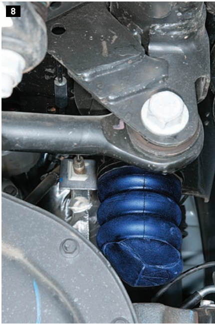
8) One-piece front spring (left) is positioned into the factory jounce bumper retaining cup. 9) Lowering the front will usually allow the spring to seat. It may be necessary to use a piece of wood to fill in the gap temporarily while seating, as was the case in the test installation (not shown). 10) The right-front factory jounce bumper (arrow) was a little more difficult to access, but it can still be done without removing the front wheels.
