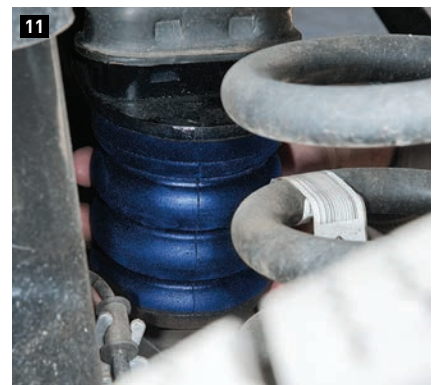
11) Once seated, the SumoSprings look like they were made for the suspension.
