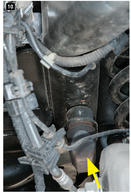
8) One-piece front spring (left) is positioned into the factory jounce bumper retaining cup. 9) Lowering the front will usually allow the spring to seat. It may be necessary to use a piece of wood to fill in the gap temporarily while seating, as was the case in the test installation (not shown). 10) The right-front factory jounce bumper (arrow) was a little more difficult to access, but it can still be done without removing the front wheels.
