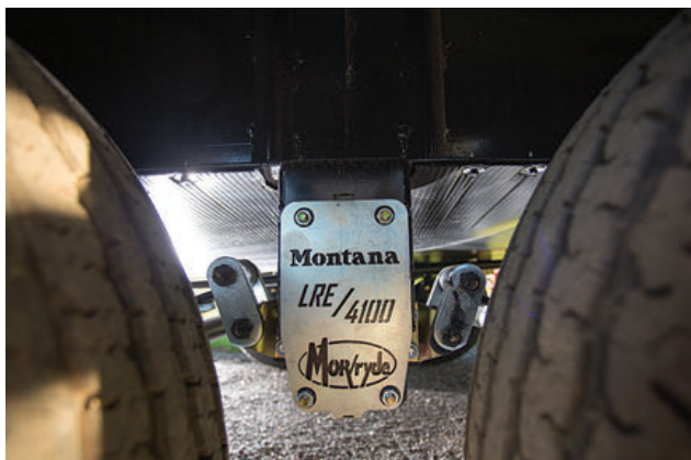
(Above) The Legacy Edition features the exclusive MORryde LRE4100 suspension, which helps smooth out the roughest road. (Above center) The front kitchen features a buffet cabinet with slide-out drawers, china cabinets and a window. (Above right) There is ample storage under the main bed in this exterior-and-interior-accessed compartment.
