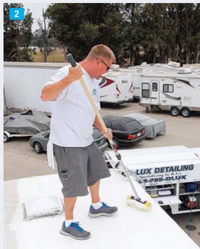
1) Keep the tip of the pressure washer a good 8 to 10 inches from the surface, passing it back and forth constantly. You can easily see how quickly and effectively it will remove ground-in dirt, but it can also damage the roof or seals if you place the nozzle too close to the surface or concentrate it in one area for too long. 2) Once done spraying an area, use the rubber roof cleaner of your choice and start scrubbing.
