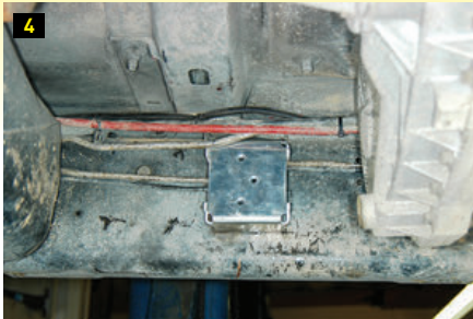
(1) Locate the original fuel filter, which is flanked by the brake master cylinder and air filter horn. (2) Original banjo bolts are on the backside of the factory fuel filter. (3) Rubber hose and new adapter fitting are connected to the fuel filter and secured with a hose clamp. (4) Instructions call for mounting the fuel pump and filter kit on the inside of the frame, but we ran into clearance problems here and elected to mount the pump on the outside of the frame (5) with the provided stainless-steel straps. (6) When using the filter kit with the BD pump, the screens are removed from the barb fitting that go into the inlet and outlet in the filter housing.
