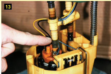
(11) After cutting the truck's fuel feed line, the rubber hose is connected and double clamped. This hose is routed to the inlet on the filter housing. (12) The fuel tank was dropped from the truck frame for access to the factory fuel basket/pump assembly. (13) The line to the original pump is lightly scored and cut at this point before removing the rest of the pump assembly. (14) The end of the fuel feed line must be cut precisely to prevent collapsing and the possibility of running out of fuel.
