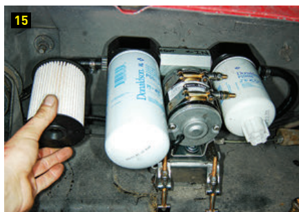
(15) The original filter on left is compared against the BD filters, one of which is a water separator. A new filter (from parts store) was installed in the factory housing at the same time. (16) A pressure switch is mounted to the CP3 rail injection pump using new adaptor and sealing washers.
