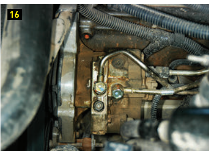
(15) The original filter on left is compared against the BD filters, one of which is a water separator. A new filter (from parts store) was installed in the factory housing at the same time. (16) A pressure switch is mounted to the CP3 rail injection pump using new adaptor and sealing washers.
