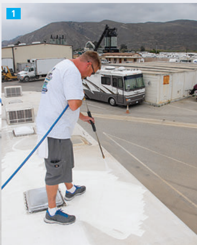
1) Keep the tip of the pressure washer a good 8 to 10 inches from the surface, passing it back and forth constantly. You can easily see how quickly and effectively it will remove ground-in dirt, but it can also damage the roof or seals if you place the nozzle too close to the surface or concentrate it in one area for too long. 2) Once done spraying an area, use the rubber roof cleaner of your choice and start scrubbing.
