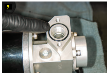
(7) Loctite gel is applied to the adapter that screws into the filter head before tightening. (8) It's important to coat the gaskets on the fuel filters so they will seal against the housings. (9) Filter fittings on the pump only use O-rings for proper sealing. (10) The pump is mounted to the frame and filter housings are attached to the pump. This is the complete assembly minus the filters.
