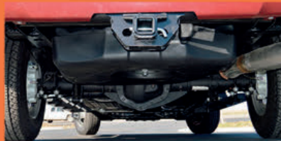
Spare Tire Auxiliary Fuel System
